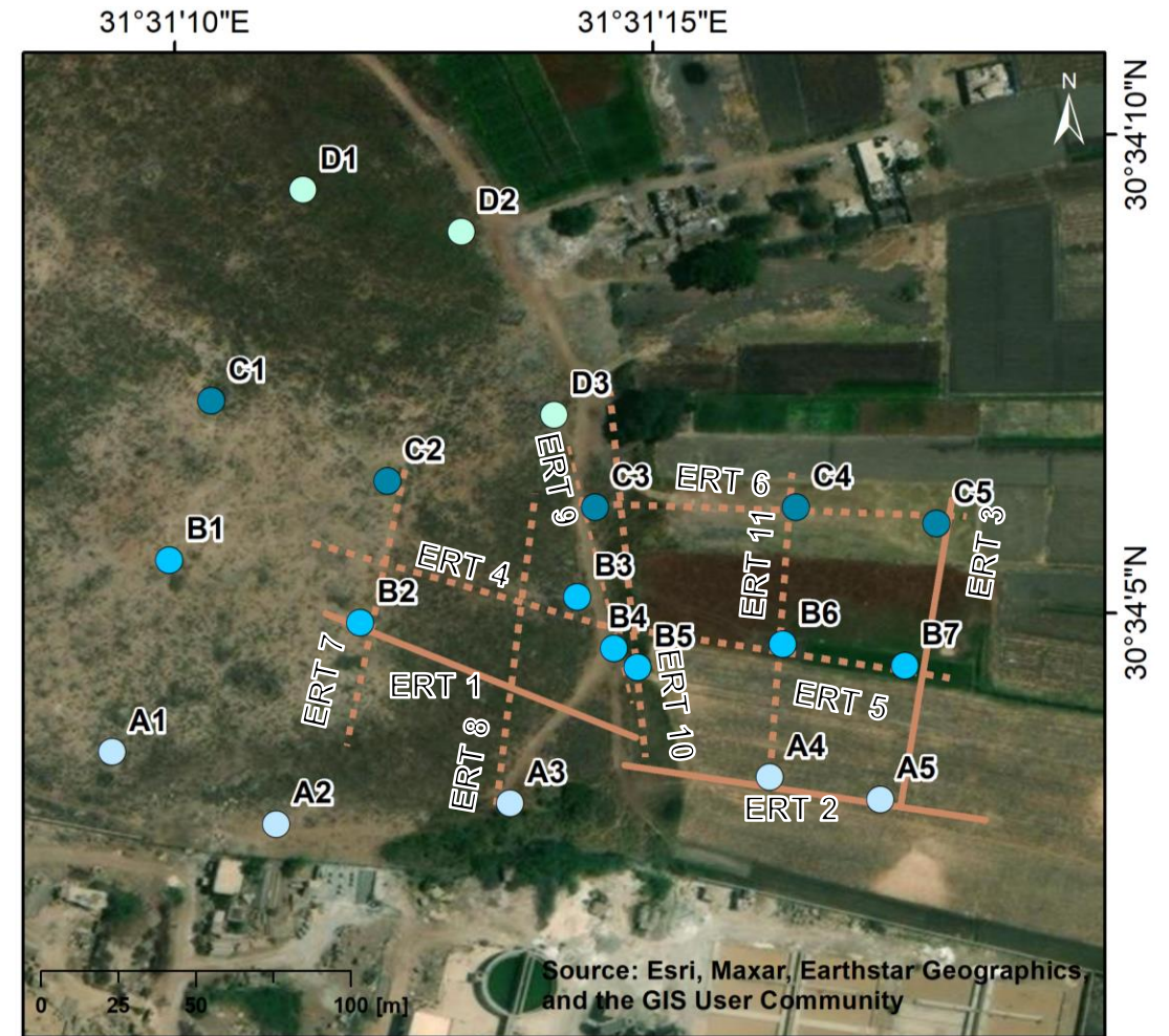
Figure S24. Overview of drilling locations and ERT profiles (only the solid ERT lines are used for the interpretation and discussion in the article).
