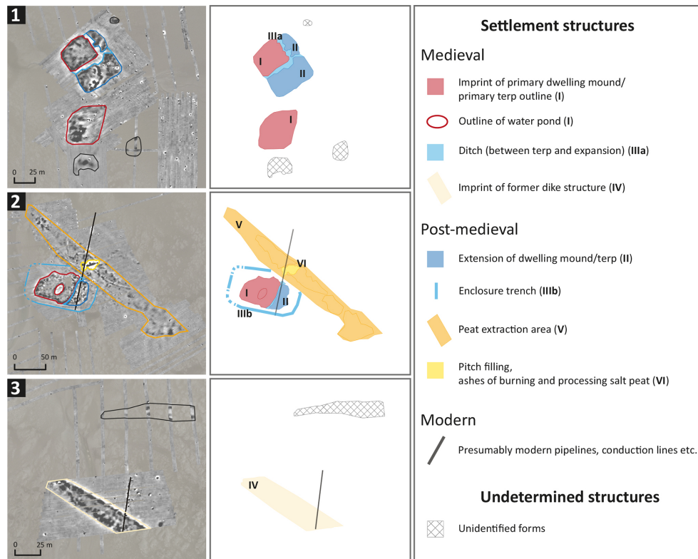
Figure 4. Interpretation of the results of magnetic gradiometry measurements and sediment cores in the study area (digital orthophotos DOP20: LVerGeo SH 2014). (1) Illustration of terp construction (I, red) and its extension (II, blue), divided by an L-shaped ditch (IIIa, light blue). (2) Imprint of primary terp base (I, red) and the terp enlargement (II, blue). The enclosure ditch (IIIb, light blue) is clearly visible south of the structures and weakly discernible towards the east. The distinctive shape of a peat extraction area (V, orange) is at a tangent to the settlement outline in the north. (3) Considering old maps and already-known dike imprints (Wilken et al., 2022), the wide linear structure is interpreted as the dike body (IV, beige) continuing towards the northwest and southeast. The anthropogenic impact in modern times is present in the form of presumed pipelines or conduction lines (black line).
