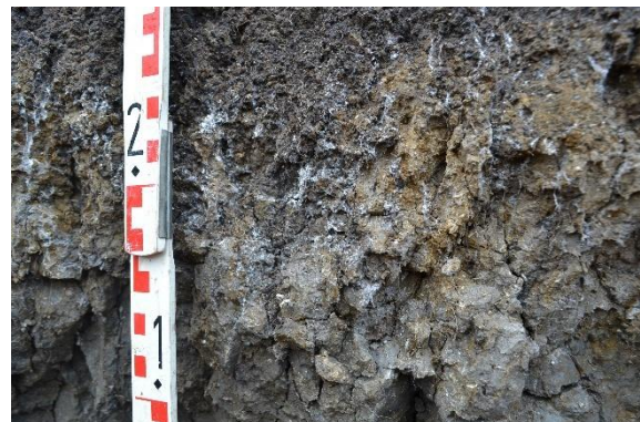
Figure S8. Unit S6 in Pit 2, characterised by excessive carbonate precipitation ( Rheinweiß ), overlain by the brown fossil top soil of Unit S5.
