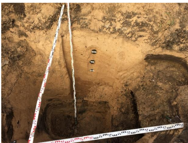
Figure S11. View from southwest onto the northeastern wall of Pit 1 with the position of OSL samples 4–6 (HDS-1821 to HDS-1823) taken in the sand infill.
