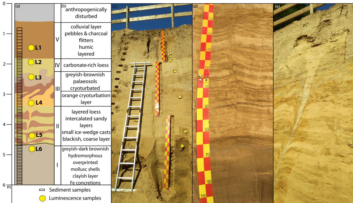
Figure 2. (a) Simplified stratigraphic sketch of the Siersdorf loess–palaeosol sequence. (b) Short description of main stratigraphic units. (c) Photo of the sequence after sampling (photo: Stephan Pötter). (d) Laminated loess package and basal palaeosol (photo: Philipp Schulte). (e) Ice-wedge cast, approx. 3 m left of the sampled sequence, piercing the underlying layers for more than 2 m (photo: Stephan Pötter).
