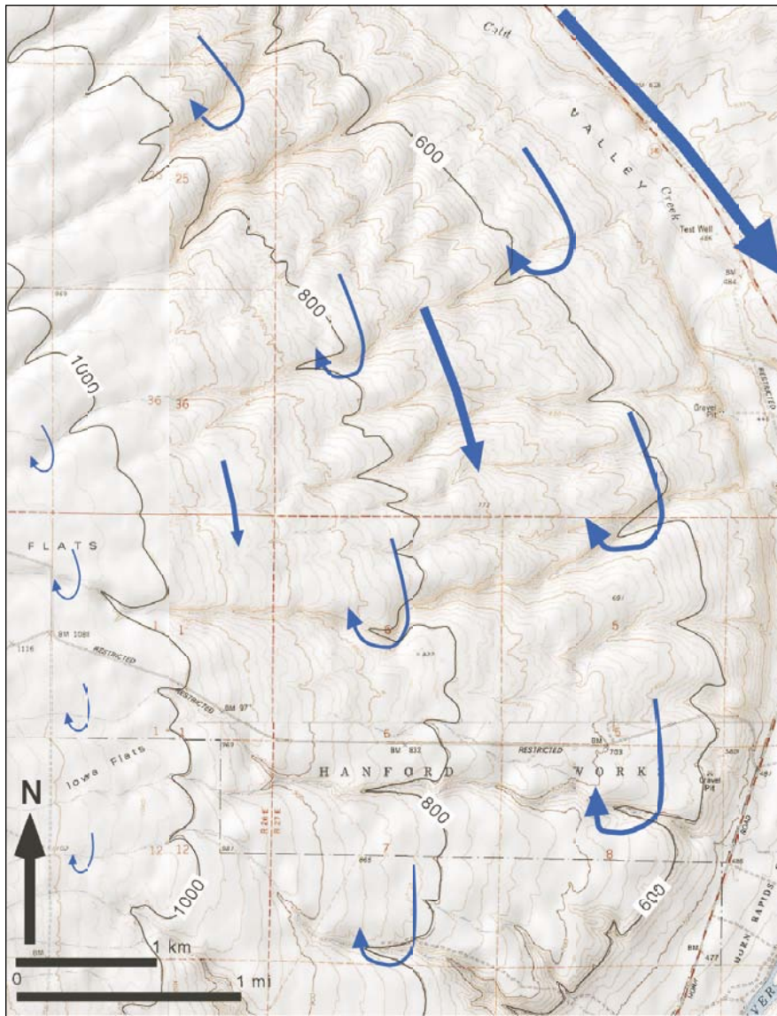
Fig. 16: Diagram showing variable flow and speed of floodwater across a portion of the study area. Where floodwaters were deeper to the right, eddy currents caused icebergs to collect and ground on upstream sides of gullies while in shallower more-restrictive waters (left side) icebergs tended to ground along the bottoms of gullies. Elevations in this standard USGS topographic map are in feet (conversion to metres = 0.3048).
